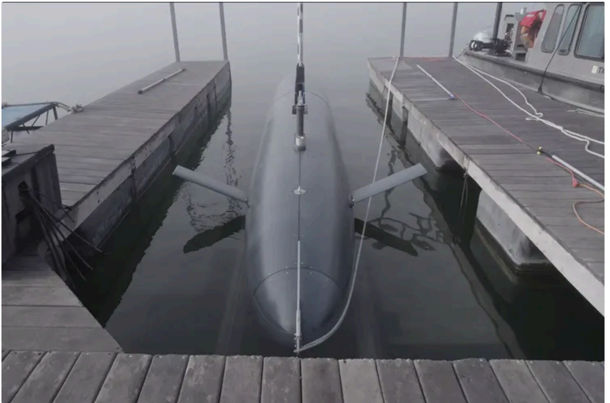
Terradepth's large unmanned underwater vehicle (LUUV) prototype in preparation for testing and development (Photo: TERRADEPTH)
